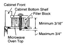
4. Insert 2 screws with washers through top cabinet holes and tighten to top of microwave oven. (While tightening screws, lift front side of microwave oven and push toward wall.)
